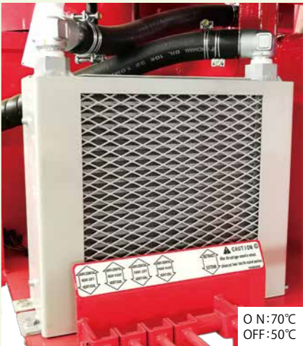
Oil Cooler (with Thermostat)
